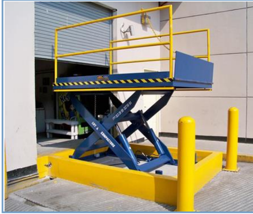
Loading Dock Lift
